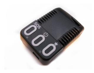
The KCS TraceME GPRS/GPS range of modules enable you to remotely track & trace a variety of objects, e.g. cars, trucks, containers, (motor)cycles. TraceME Micro is the latest addition, targeted for personal use and any other application that need a minimum size while maintaining the exact same options and server connection the full-size units have.
